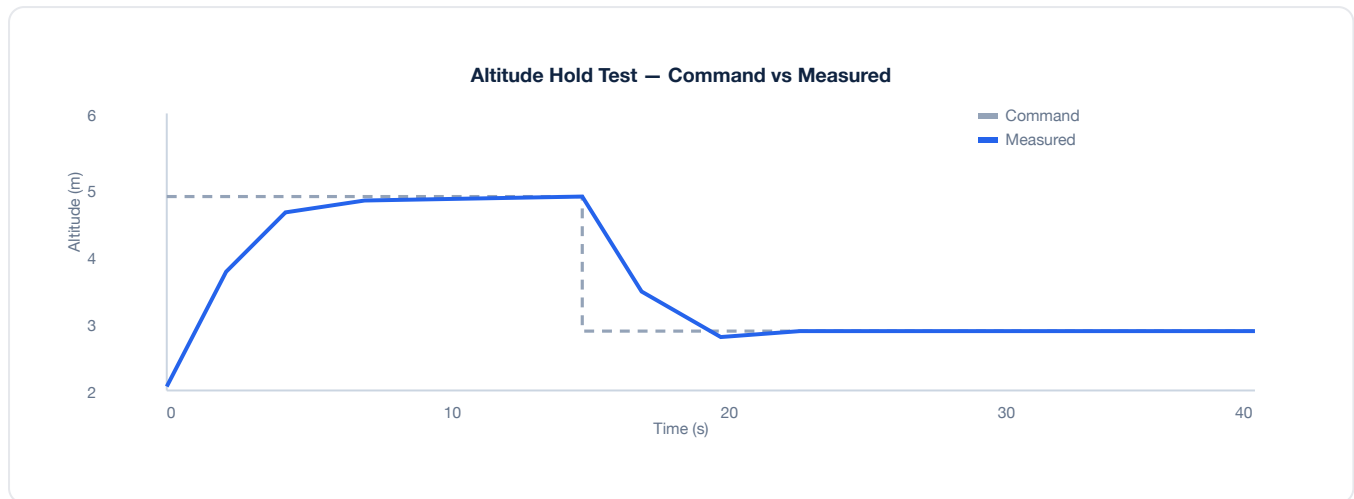
Figure 2. Altitude hold: measured altitude against the commanded step (5 m \rightarrow 2.5 m). Settling time \approx 5 s, steady-state error < 0.1 m; overshoot below 5%.
