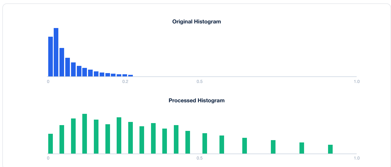
Figure 3. Histogram analysis: (top) the original V-channel pixel values are compressed into [0, 0.2]; (bottom) after processing the values are spread evenly across the full [0, 1] dynamic range.
