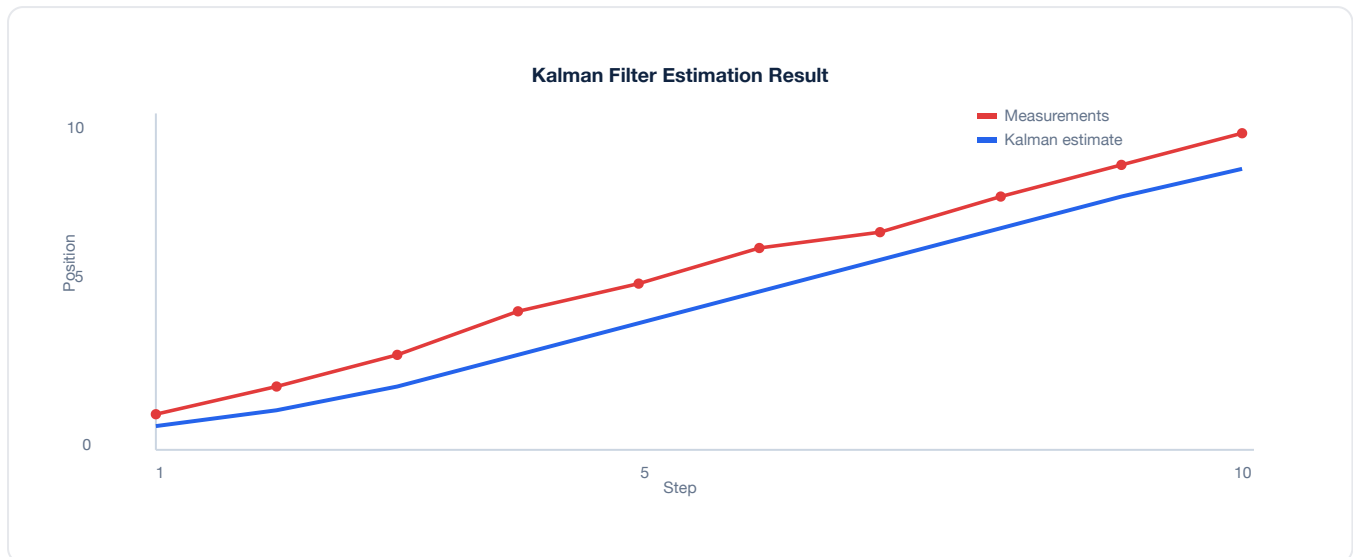
Figure 6. Kalman filter result: red = noisy measurements, blue = the filter's estimate. Despite high measurement noise, the state is tracked successfully.
